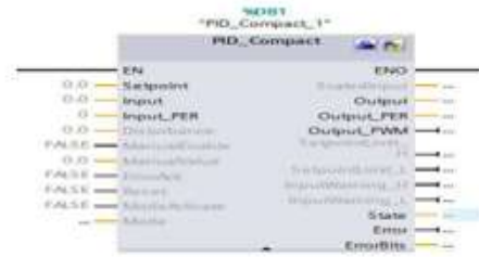
Figure 4.4: Working block diagram of PID_Compact PLC S7-1200
